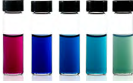
Figure 23.5: Different color fluids containing nano-particles can be obtained by changing the permittivity of the background fluids (courtesy of nanocomposix.com).
